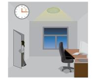
Light will dim to 10%/20%/30%/50% (options) after the hold time when no movement in detection area
